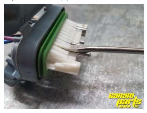
with the screw driver inserted pull the wire out.
