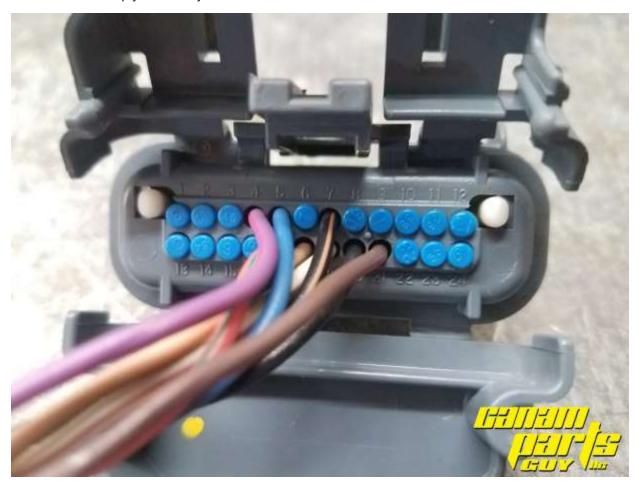
2008-12 wire layout bottom row showing the colors and numbers Double check your lay out and re assemble the machine, you may have to plug in with BUDS to pair the new dash with your machine.
