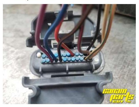
This smoke color guard needs to be removed there are two tabs that need to be depressed for it to slide off.
