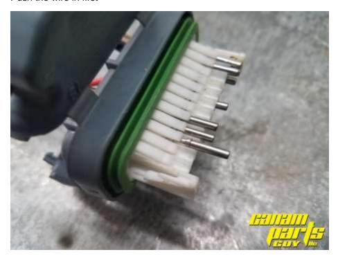
using the small screw driver pry up the plstic clip
